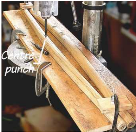
▲ Pic. 2 Here you can see the set-up for drilling the seat rail mortise holes
